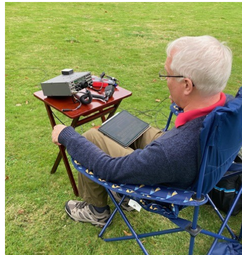
Paul M1CNK used an end fed half wave on the HF bands, with SSB from his K2 and data (FT8) from his QMX
