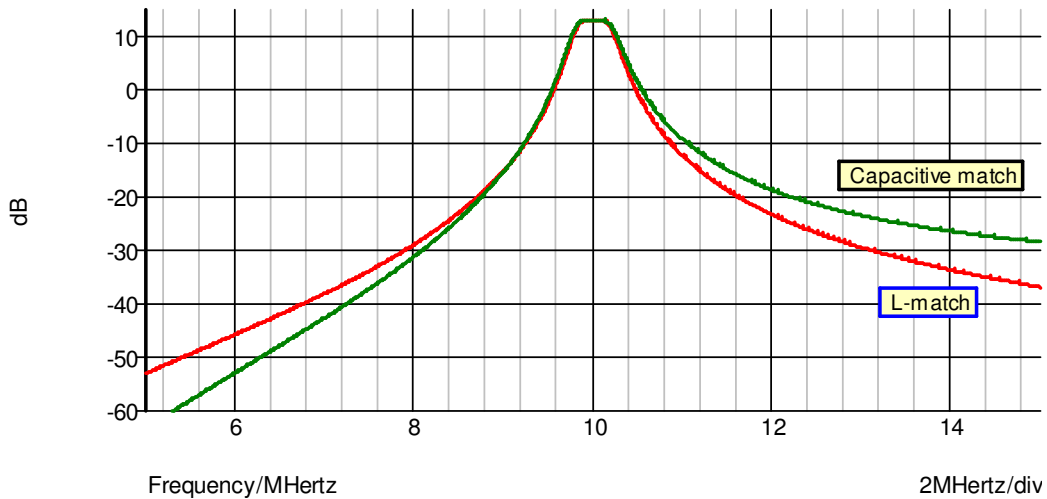
Fig. 9. Comparison of L-match and capacitive match
