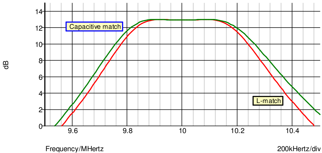
Fig. 10. Comparison of L-match and capacitive match – pass band response
