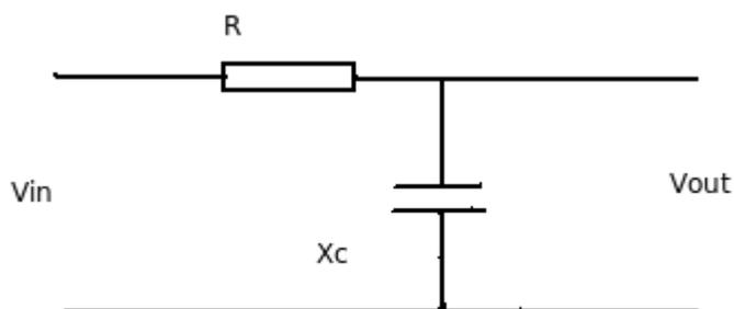
This will be recognised as a 1<sup>st</sup> order low pass filter. So what are the steps to get an equivalent performance implemented as algorithm on a computer?
