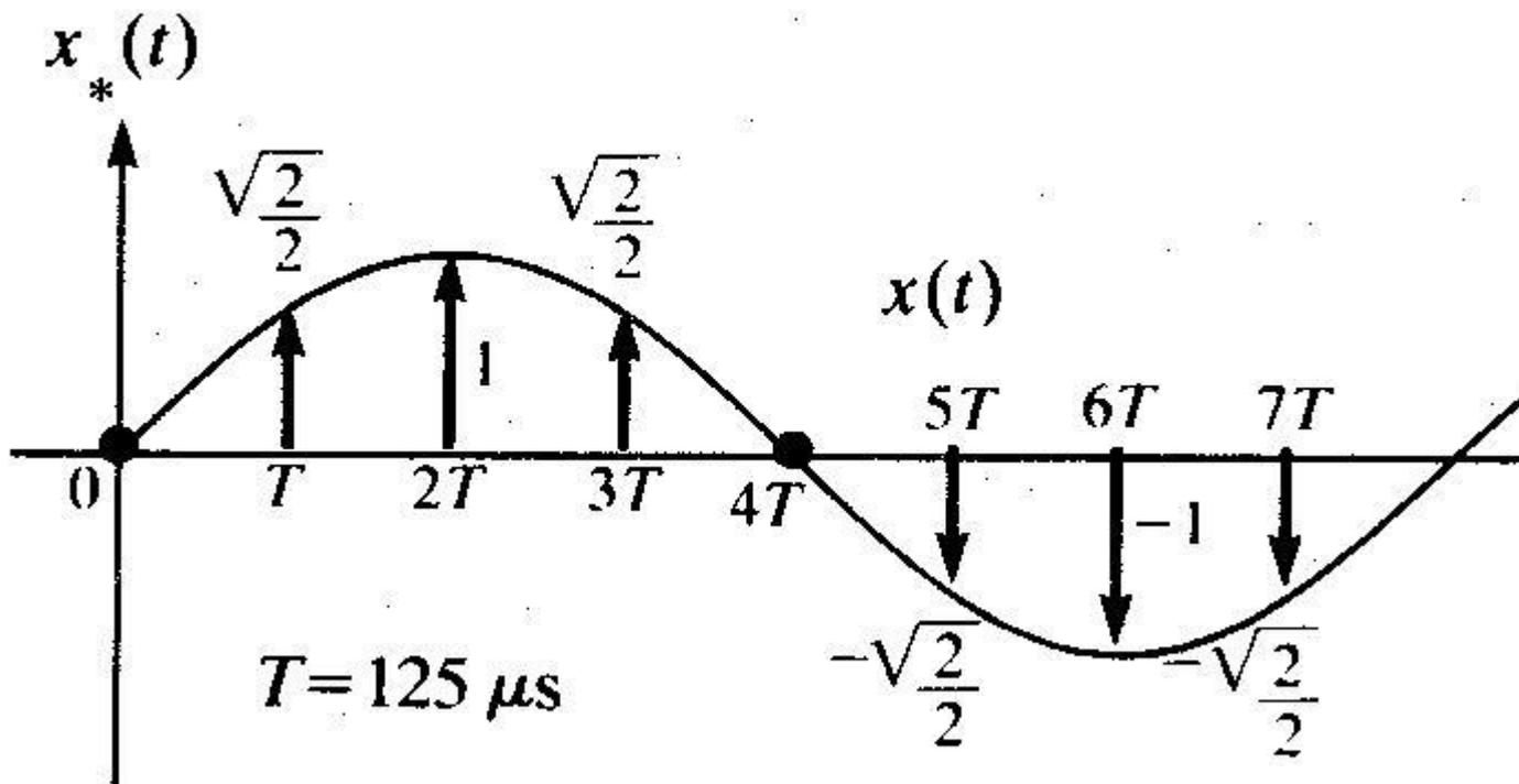
Fig 5.1 Sampled sinusoid ( Open University)
