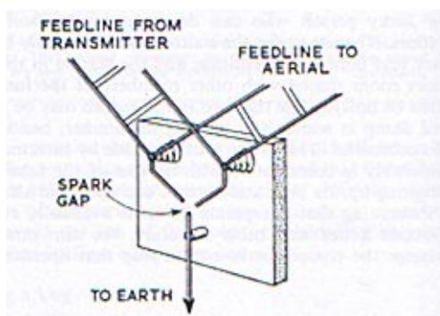
**Fig.5 Spark gap for open wire feeders (RSGB Handbook)**
