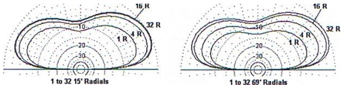
**Maximum Gain Elevation Patterns: 69' Base-Fed Inverted-L With Different Size Radial Sets**
