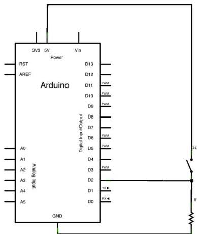
For `pinMode(INPUT_PULLUP)` an  $20\text{k}\Omega$  resistor internal in the Arduino holds the pin at 5v, so no external resistor is needed
